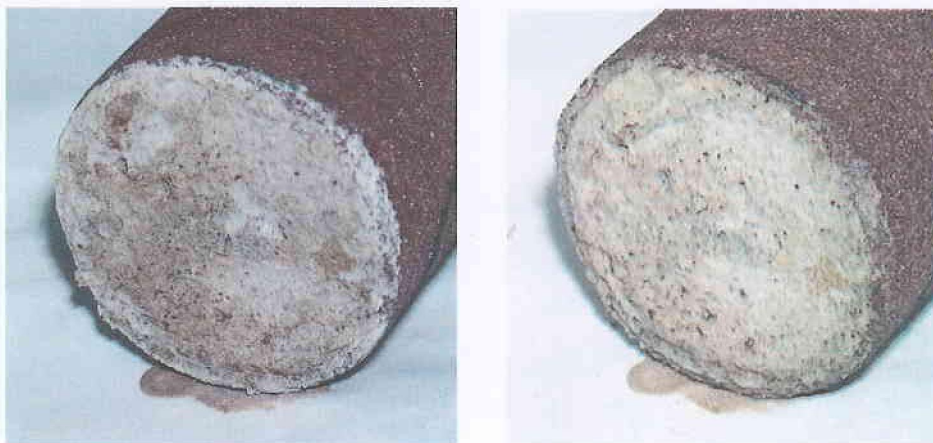
Fig. 3. Images of sample No. 1 after exposition on drilling mud and after final measurement of permeability
