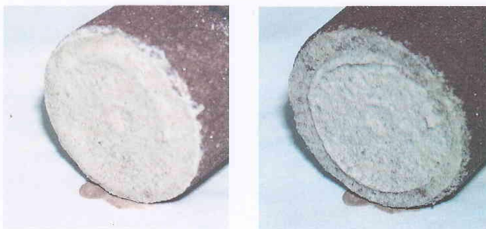
Fig. 4. Images of sample No. 2 after exposition on drilling mud and after final measurement of permeability
